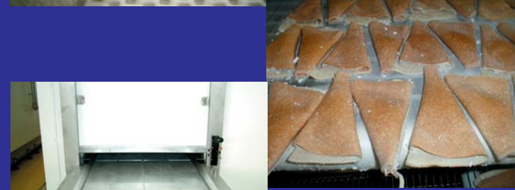
It also enables unpacked sensitive products to remain flat and unmarked, Example opposite : coated products or below : frozen filled crepes.
