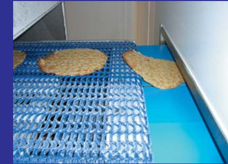
This model is also used for products requiring a very short passage and a very rapid conveyor time such as crepes (30 seconds).
